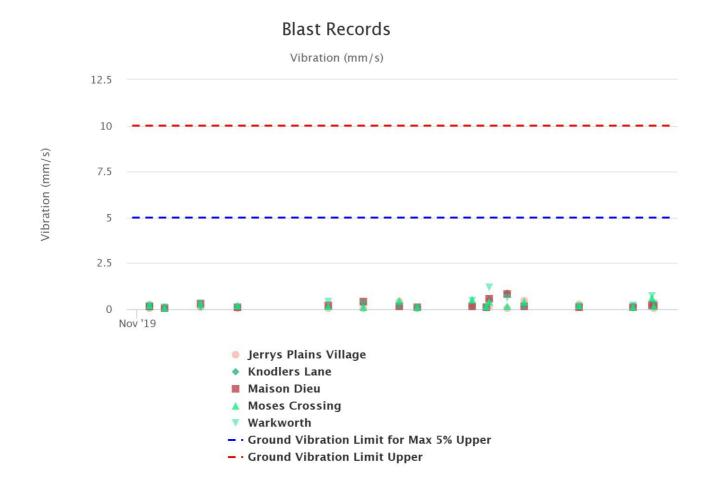
Figure 11: Ground Vibration Blast Monitoring Results – November 2019
