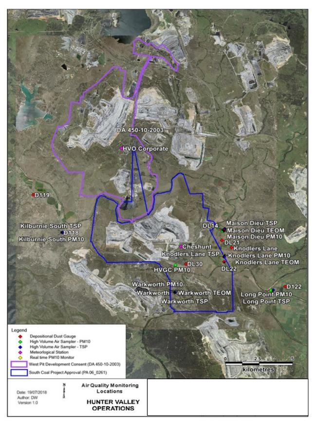
Figure 4: Air Quality Monitoring Location Plan
